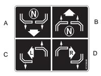
The steering levers control speed and direction. In addition, they will stop the unit.
